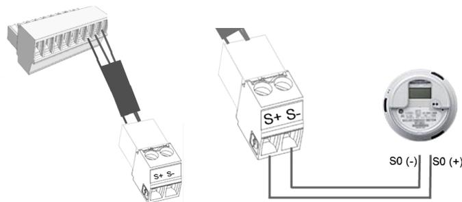
Figure 11: S0 meter connection to the S0 adapter cable
