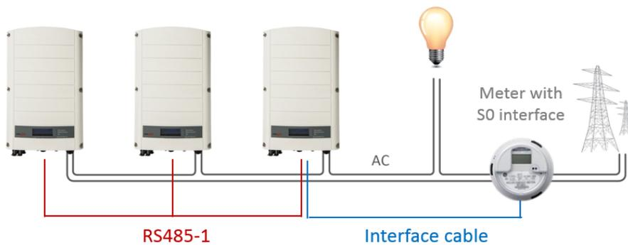
Figure 7: Multi-inverter connection with S0 meter and RS485 communications
