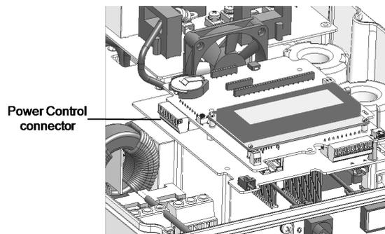
Figure 12: Inverter communication board
