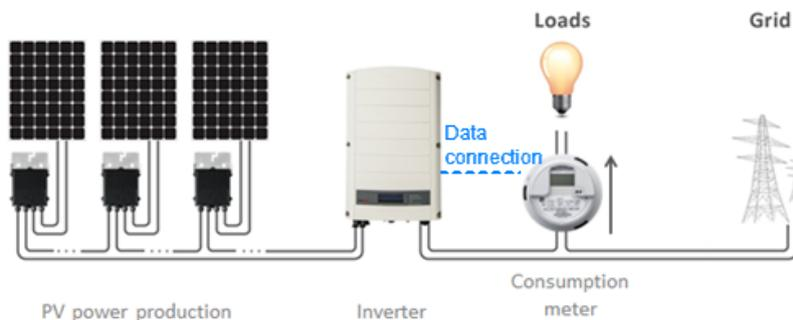
Figure 3: Typical installation with meter measuring consumption
