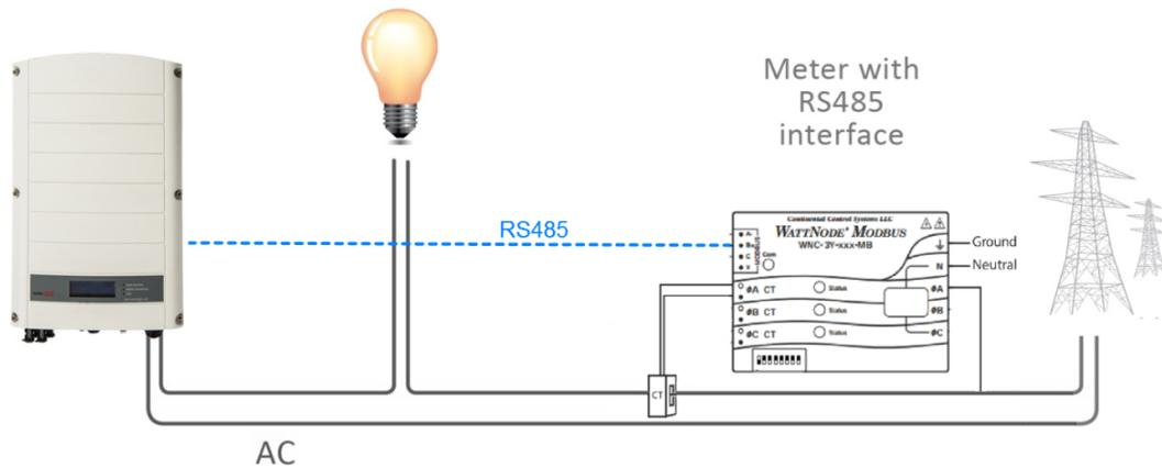
Figure 4: Single-inverter<sup>1</sup> connection with RS485 meter<sup>2</sup>
