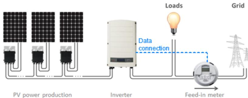
Figure 2: Typical installation with meter measuring feed-in
