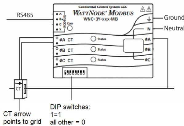
Figure 15: Meter Connection diagram
