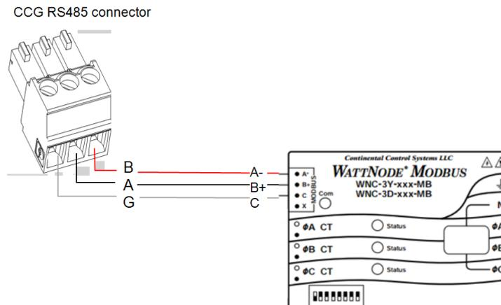
Figure 9: WattNode meter connection to the CCG RS485 connector
