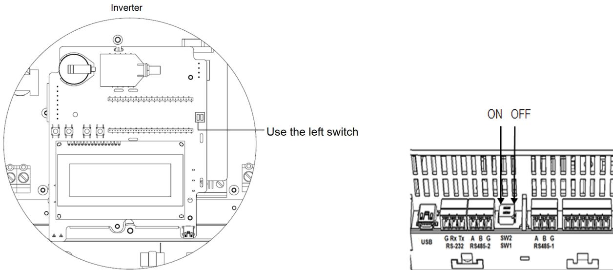
Figure 17: RS485 termination switch
