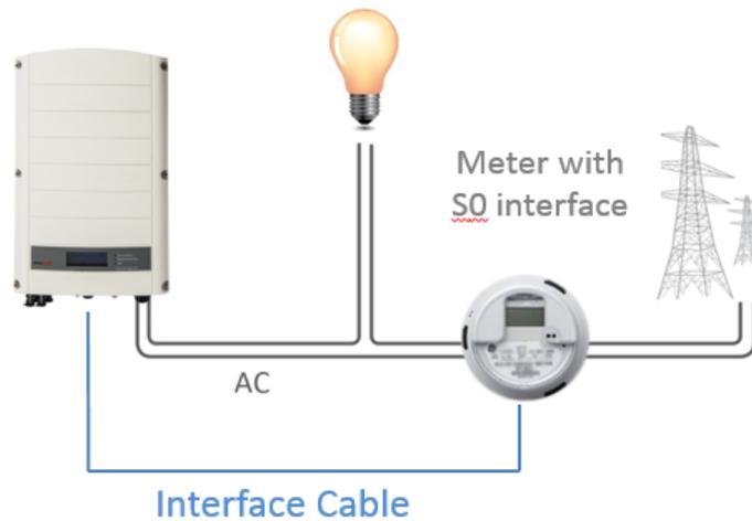
Figure 5: Single-inverter connection with S0 meter
