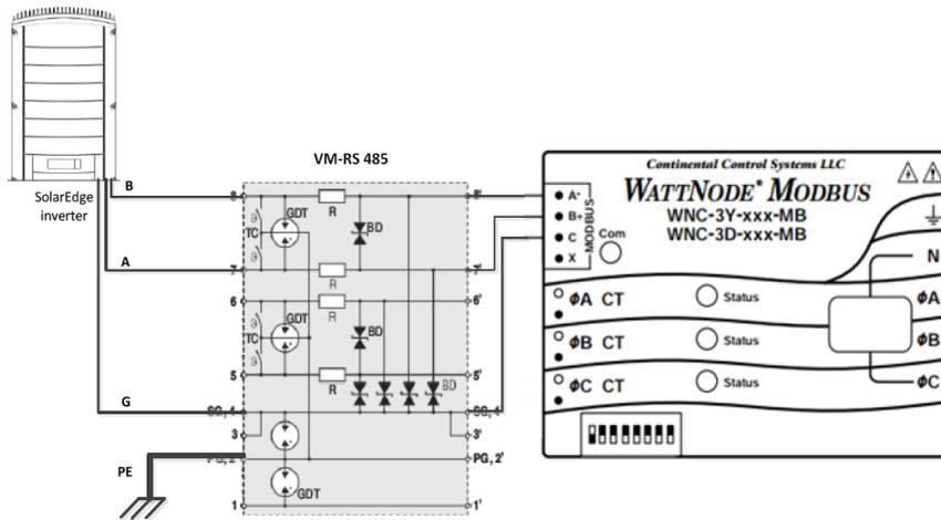
Figure 18: Protection connection
